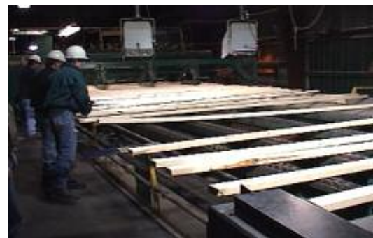
Finished Lumber Grading Station
